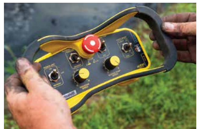
Control a radio de la Draga Crisafulli FLUMP.
